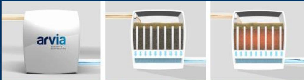
Figure 2. Modular design of Arvia's Nyex™ treatment system which treats water by adsorbing organic contaminants from the influent as it percolates the packed bed of Nyex™ particles, and the simultaneous passing of current ensures in situ oxidation of the adsorbed organic.
